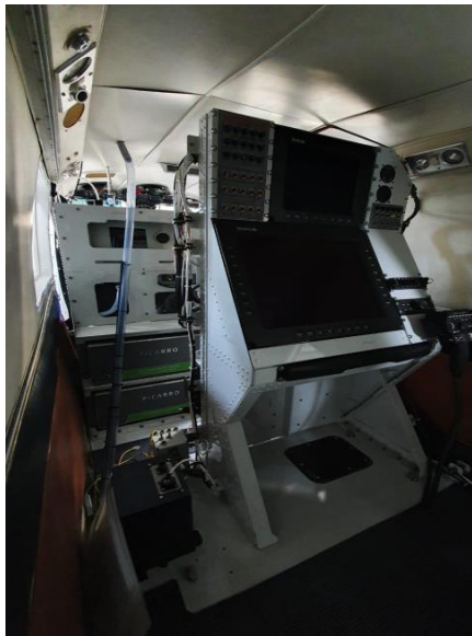
Figure 30. Picarro G2401-m onboard BN2A-27 (left) and the working principle (right)
