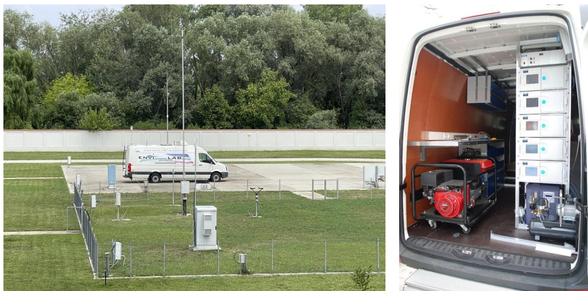
Figure 25 Van with HORIBA monitors measuring during QA4EO campaign at MARS site in Magurele
