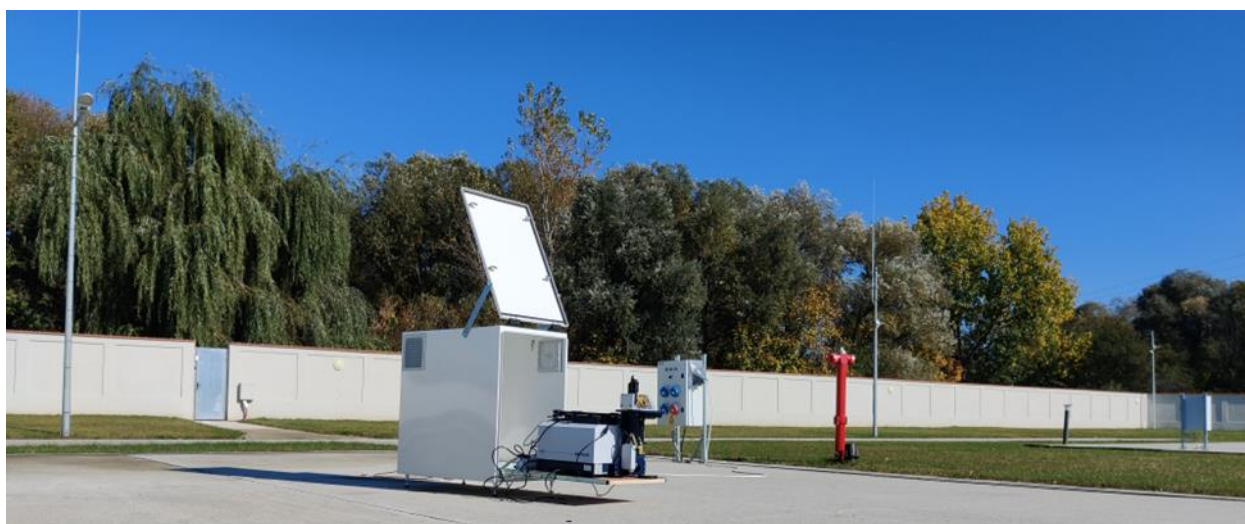
Figure 24 EM27/SUN spectrometer taking measurements at MARS, in Magurele
