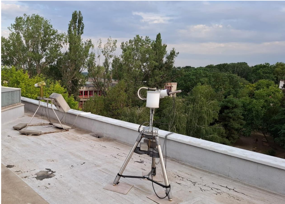
Figure 23 Pandora - 2S left side, near the sunphotometer -right side of the picture on the rooftop of RADO in Magurele
