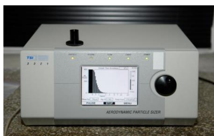
Figure 32. Aerodynamic Particle Sizer (left) and its installation aboard INCAS BN2A-27
