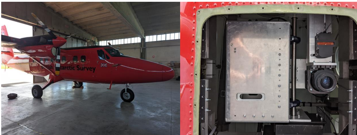
Figure 79 BAS Twin Otter (left) and SWING scanner integrated in the bottom plate alongside the SPECIM OWL spectrometer (right) (25/05/2023, Siena Aerodrome).
