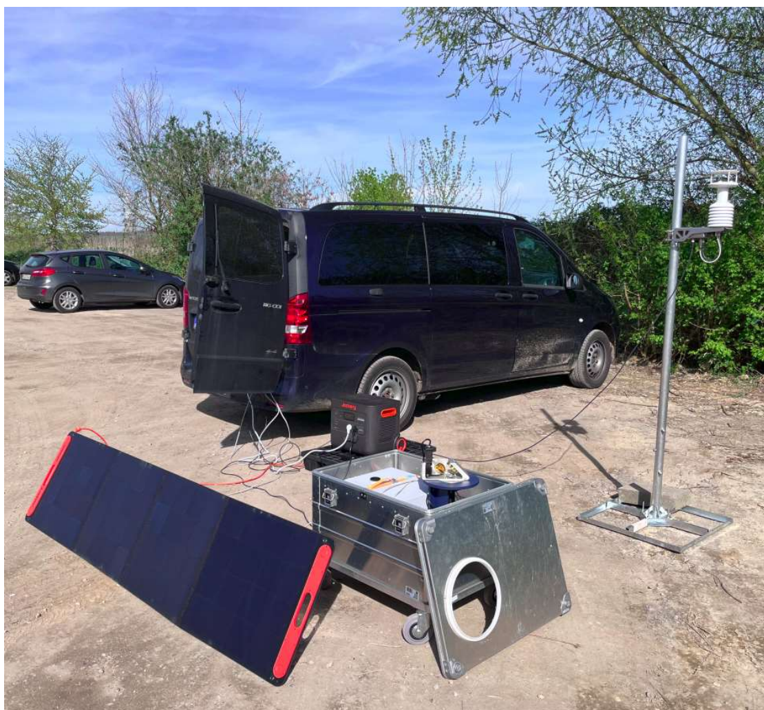
Figure 1 Bruker EM27/SUN spectrometer with compact solar tracker and Gill MetConnect One weather station at location Wed.3. A portable battery and solar panel provide power for the measurements in the field.
